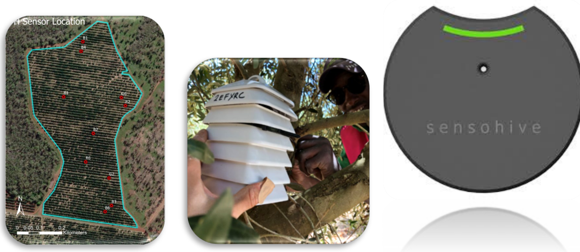
Figure 11. Locations of canopy sensors placed on one of the Bundaberg farm 1 blocks; the steveson screen attached to the trees and Sensohive RH and Temperature sensor.
