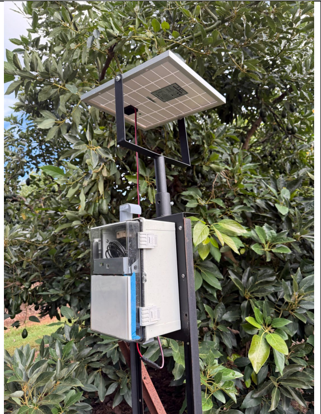
Fig 1.2 – Installation of camera housing (enclosed camera, electronics, battery), and solar panel mounted on top. Custom fabricated metal setup.
