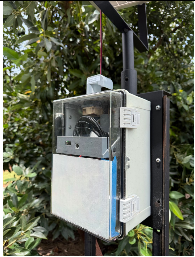
Fig 1.5 – Close up of the camera enclosure.
