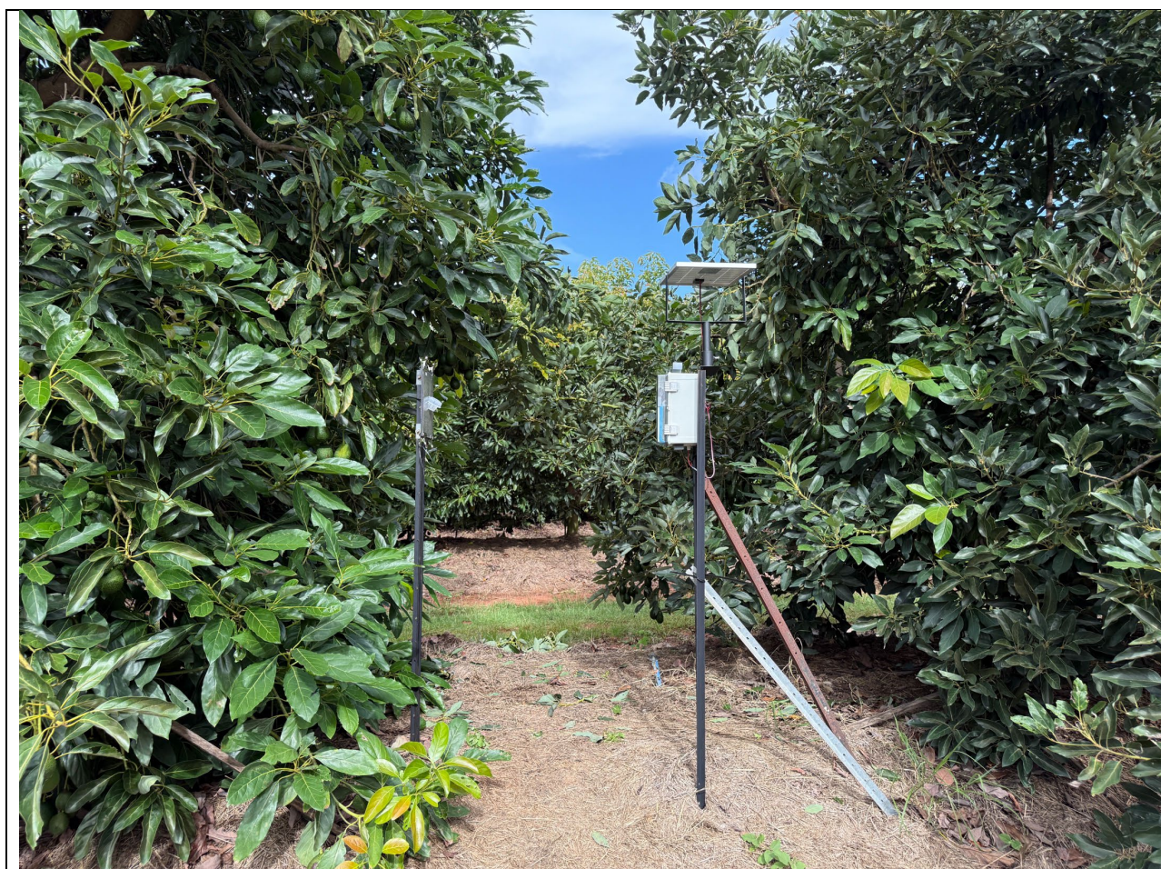
Fig 1.3 – Installed lure and board (left), and the AI camera system (right). Approx 1m apart. Overhead branches cleared to improve solar access.
