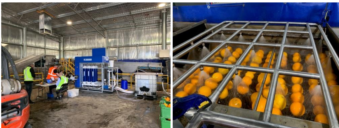
Figure 27. The trial Unipolar® EW system in the commercial packinghouse (left) and treatment of oranges with Unipolar® sanitiser over brushes (right)
