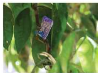
Water sensitive papers (WSP) are pinned to leaves inside and outside the canopy.
