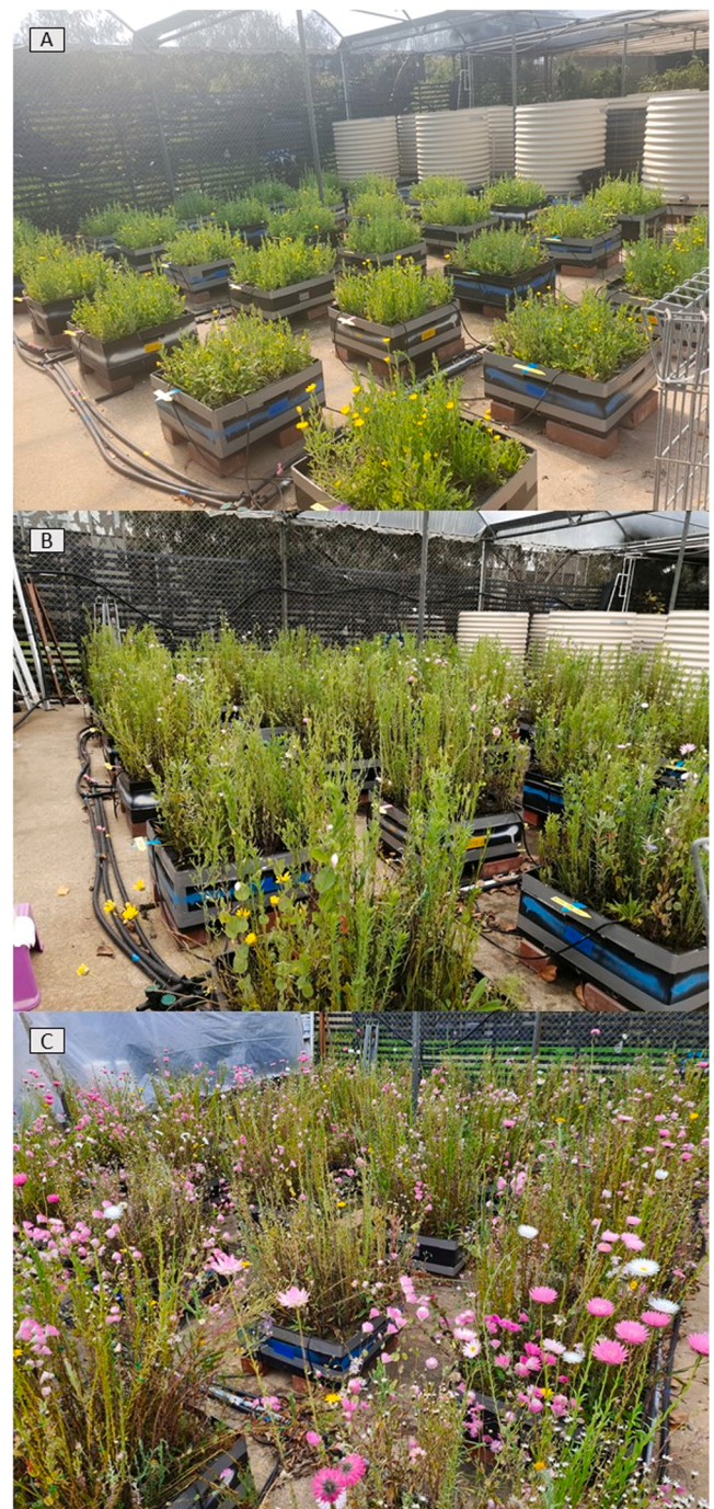
Fig. 2. Green roof modules at the experimental site of University of Melbourne, Burnley Campus, three (A), six (B) and nine (C) months after sowing (April, July, Sep 2020, respectively).
