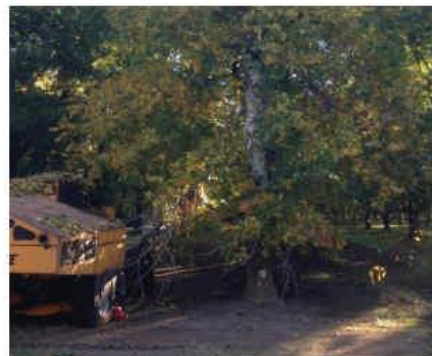
Tree shakers are used to shake mature nuts from the trees. Trees are shaken for between 3 and 5 seconds and mature nuts fall to the ground.
