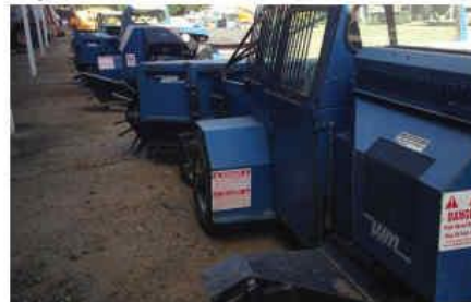
Sweepers sweep nuts into a windrow using machines that have a rotating front sweeper and side blower.
