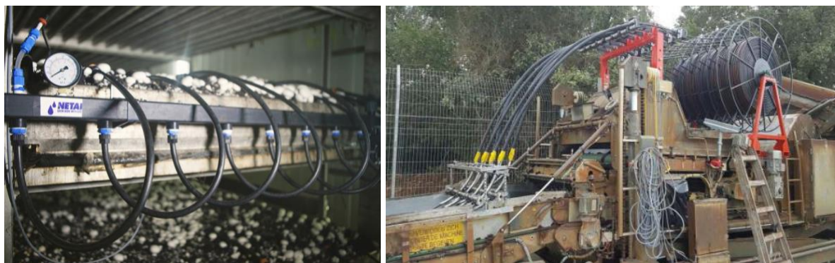
Figure 3. The Netafim "Mushroom Master" drip irrigation system (left) and the insertion unit on a Thilot head filler. From Raz et al., 2016.
