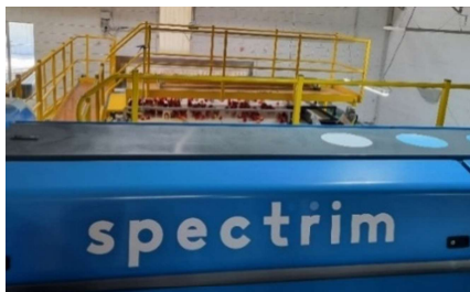
TOMRA Compac apple grading machine - Spectrim
