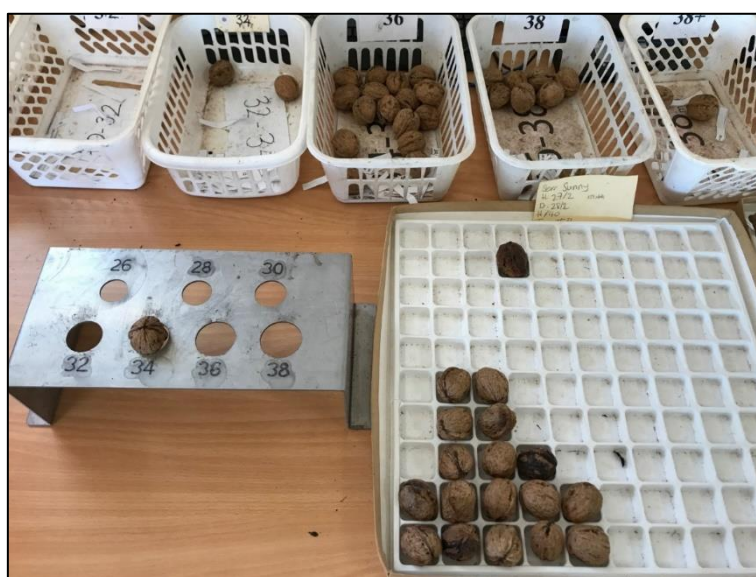
Figure 3.5. The equipment and set up used for sizing component of the walnut quality assessment
