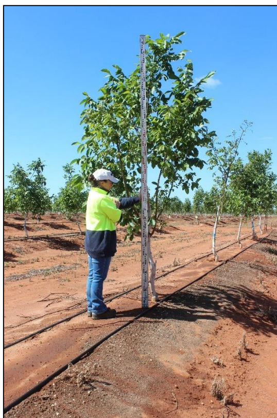
Figure 3.2. Tree heights were measured using a telescopic measuring pole.
