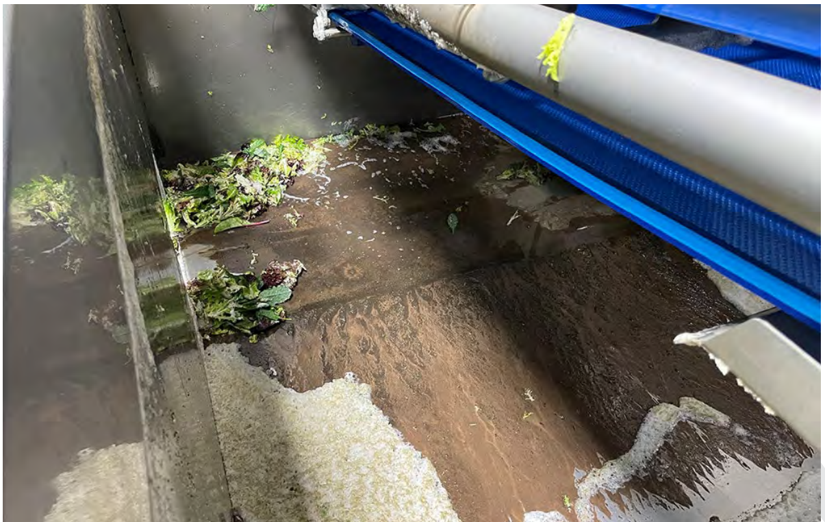
Figure 47. Accumulation of residual soil and organic matter at the bottom of a wash-water tank following the harvest of baby spinach after heavy rainfall.
