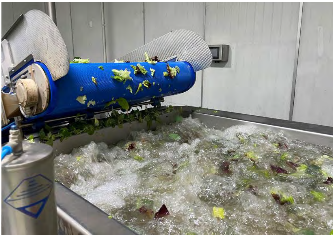
Figure 56. The wash water must have appropriate sanitiser concentrations.
