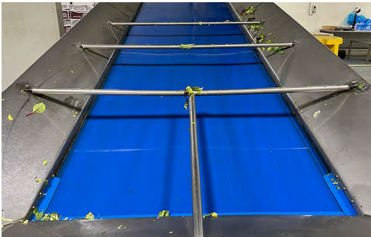
Figure 35. Removal of plant debris and organic matter from processing equipment during cleaning is essential to ensure effective sanitisation and reduce the risk of microbial contamination.
