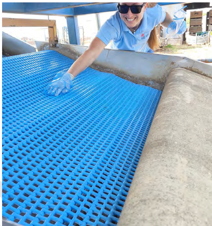
Figure 34. Environmental swabbing of harvesting equipment to verify the effectiveness of cleaning and sanitisation.
