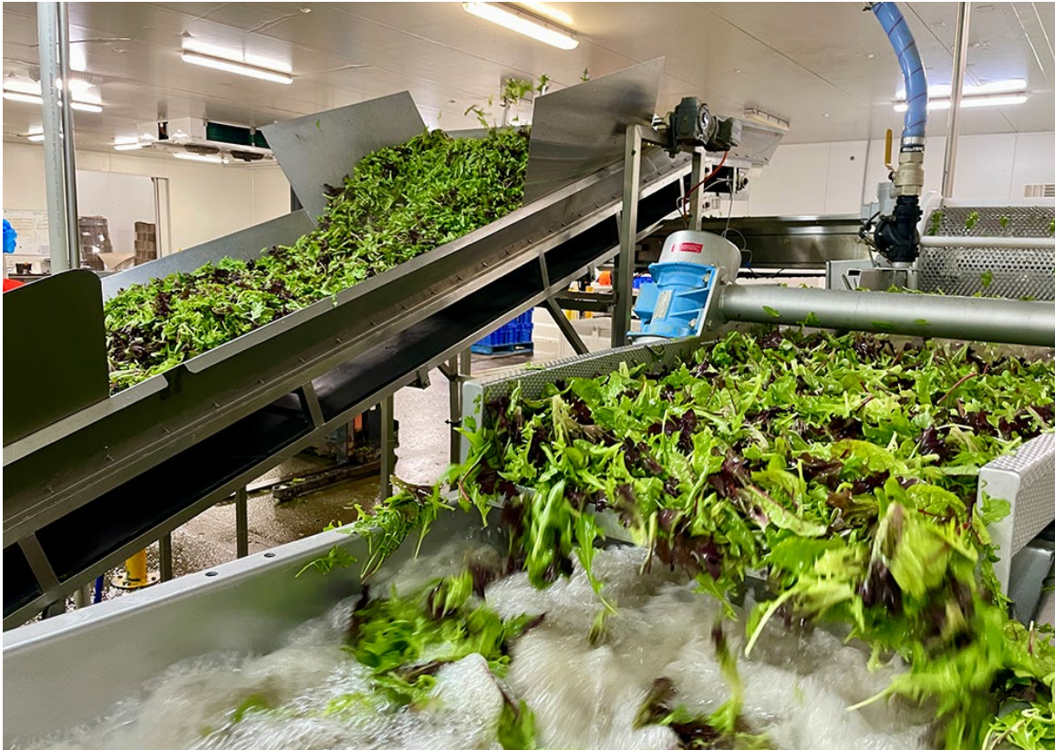
Figure 7. Appropriate sanitiser concentrations should be in each washing and sanitising tank.
