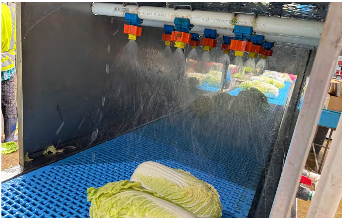
Figure 49. Spray washing Chinese cabbage (wombok) on a conveyor belt before packing.
