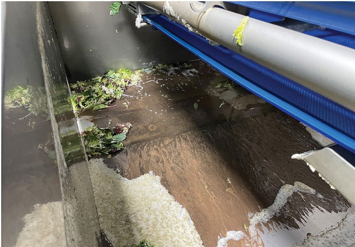
Figure 48. Accumulation of residual soil and organic matter at the bottom of a wash-water tank following the harvest of baby leaf after heavy rainfall.
