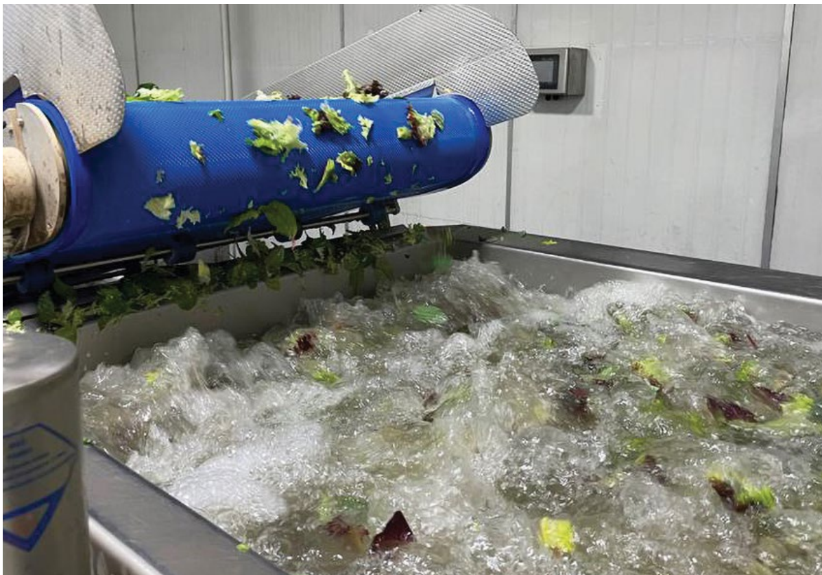
Figure 67. The wash water must have appropriate sanitiser concentrations.
