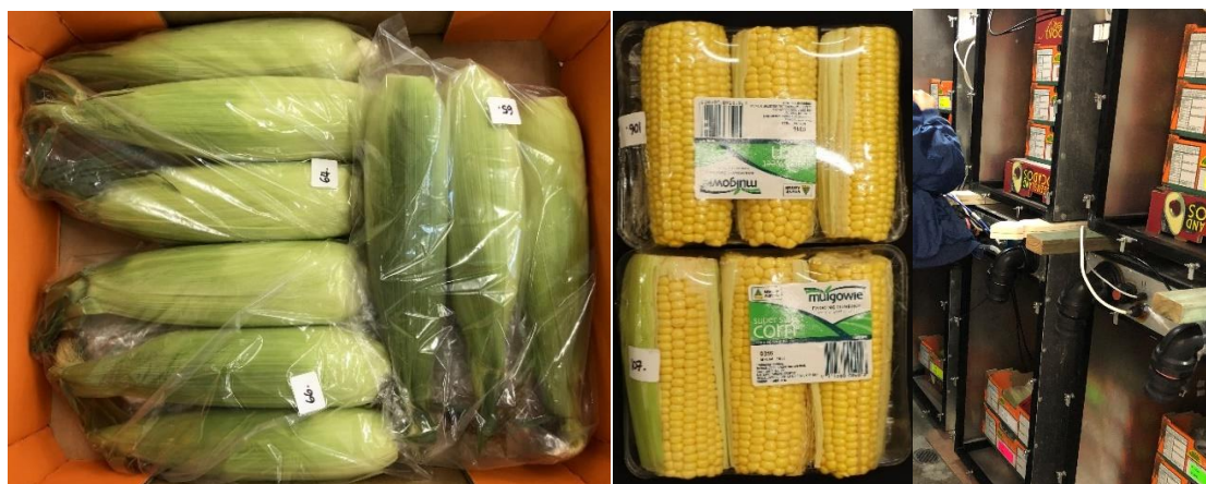
Plate 2. Sweetcorn packaging types tested in experiment 1: fully husked cobs wrapped in perforated bag (left) and semi husked cobs wrapped in cling film around a plastic tray (middle). Samples were placed into experimental chambers (right) for storage under either CA (top three chambers) or air conditions (bottom three chambers).
