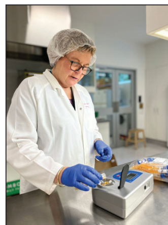
ONE OF THE QUEENSLAND DEPARTMENT OF AGRICULTURE AND FISHERIES (QDAF) CONSUMER SENSORY TEAM POURING ROCK MELON JUICE INTO A BRIX METER. THE QDAF TEAM CARRIED OUT OVER 4,000 BRIX MEASUREMENTS DURING THE CONSUMER TASTE PANELS.
