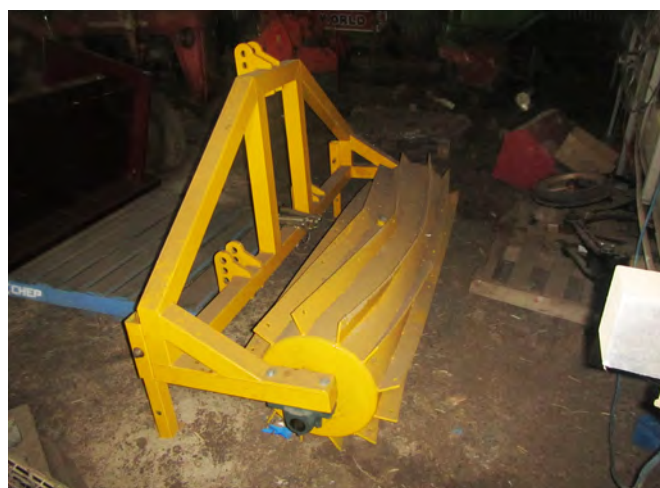
Figure 3-31. This crimping roller is used on an organic vegetable farm to prepare a killed mulch for the subsequent cash crop to be planted in to (Location: Gatton, Queensland).
