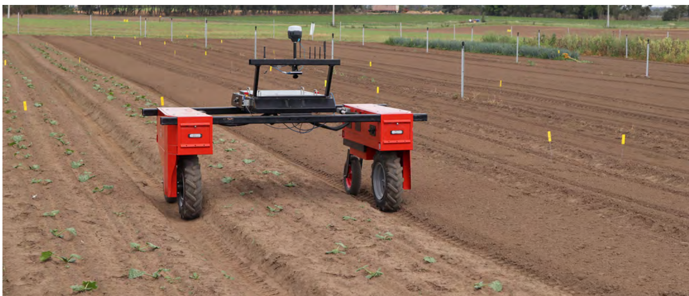
Figure 3-43. This field robotics device, developed by the University of Sydney and Agerris, is designed to carry out non-chemical weeding and intelligent spraying through weed detection sensors (Location: Richmond, New South Wales).
