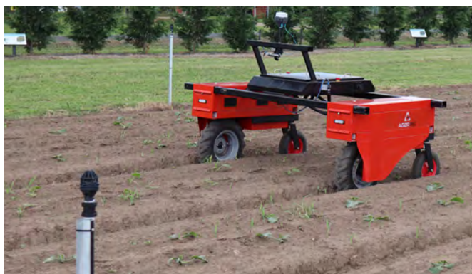
Figure 2-9. The Digital Farmhand, developed in Australia by Agerris, is one of several robotic systems under development for automated completion of a variety of farm management activities, including precision weed management (Location: Richmond, New South Wales).
