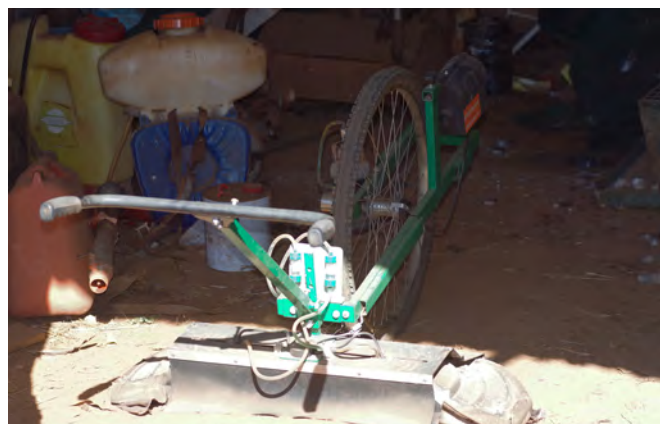
Figure 3-6. Mankar hand-operated low volume shielded herbicide applicator used with a non-selective herbicide to manage inter-row weeds at a market garden farm (Location: Moriarty, Tasmania).
