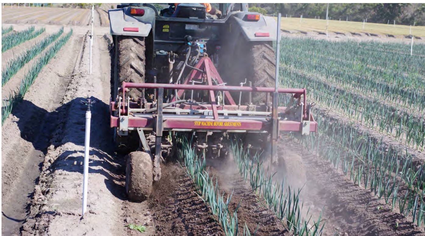
Figure 3-15. Weedfix cultivator used for inter-row tillage near Clyde, Victoria. This photo illustrates one of the benefits of inter-row tillage. By 'hilling' a little soil into the plant rows, the tillage pass may be covering and suppressing growth of some recently germinated weeds.
