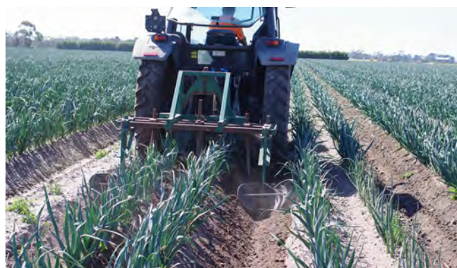
Figure 3-14. Customised inter-row cultivator used for inter-row tillage in a leek crop near Clyde, Victoria. Note that the implement cultivates both the wheel tracks and the sides and centre of the raised crop bed.
