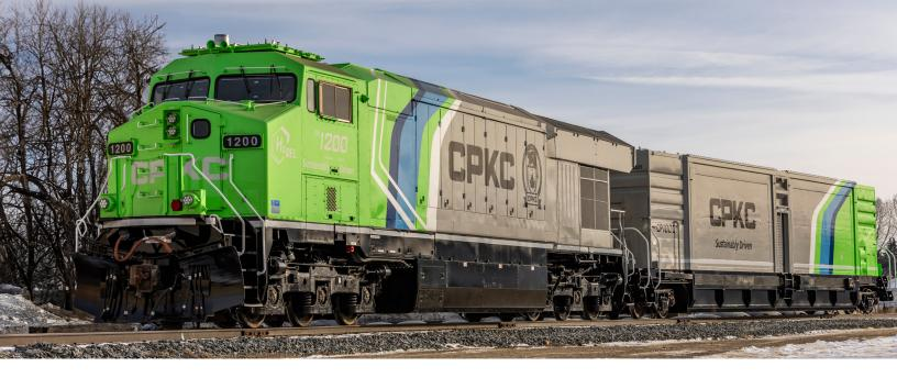
A hydrogen locomotive generates electricity using its fuel cell. It also generates electricity using regenerative braking, in which it absorbs the train's downhill momentum, powering a generator while it keeps train speed under control. Electricity from these two sources charges banks of batteries carried onboard the locomotive. The batteries then feed electricity to the locomotive's traction motors.
