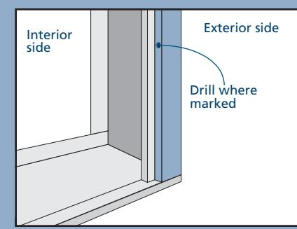
4. When painting or finishing, make sure the plunger holes are not filled with paint that will restrict operation.
