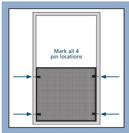
2. Remove the screen and drill a 1/4" diameter x 1/4" deep hole in the center of the exterior stop area at each mark.
