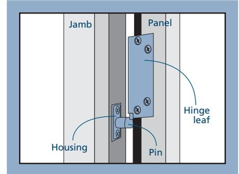
6. Slide the top hinge leaf onto the upper pivot and align the top of the panel with the hinge leaf. Fasten the leaf to the door panel with the #10 x 1½" flat head screws.
