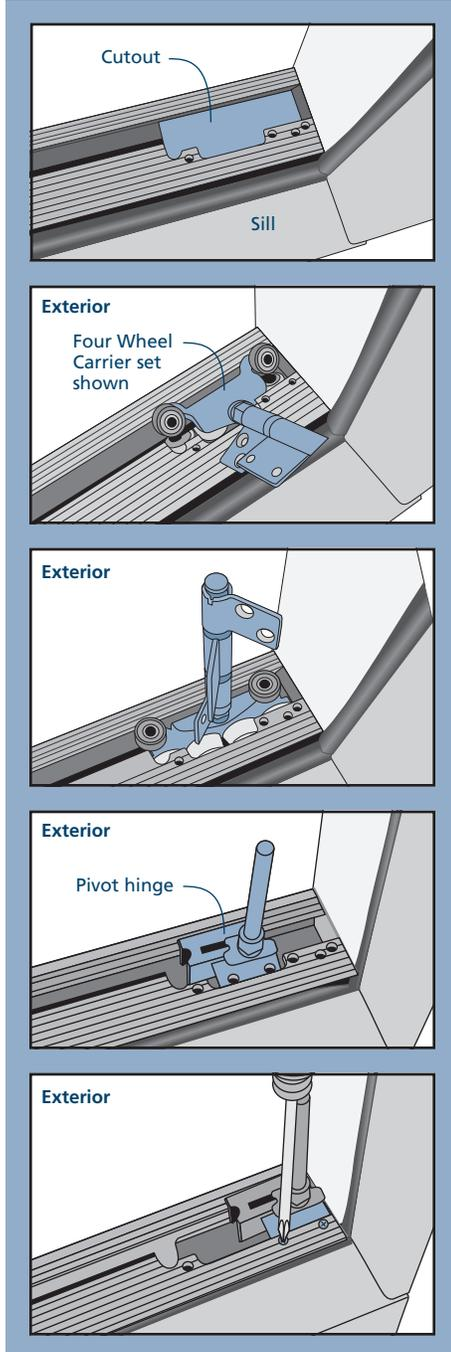
4. Insert the properly handed pivot hinge. Hinge should be inserted so that the heel, with the two screw holes, is towards the interior of the sill track. Slide all the way against jamb.
