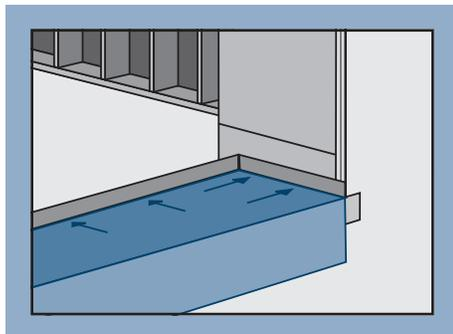
5. Cut two pieces of self-adhered flashing 9" wide by the sill pan width + 3" long.
