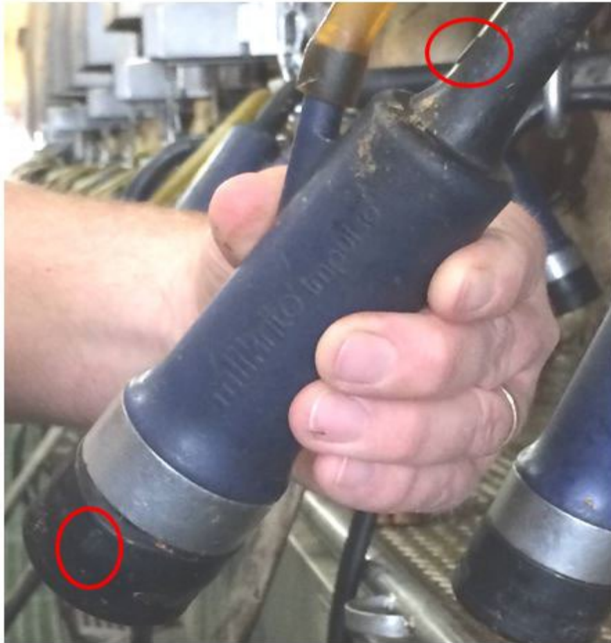
Fig. 1; Hash marks (red circles) should be aligned with one another, the 90 degree difference indicates a twisting of the liner within the shell
