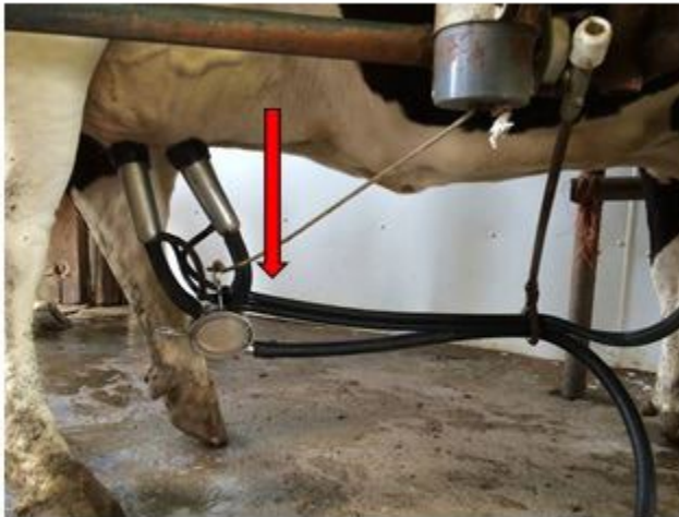
Fig. 4; Milking unit should be perpendicular to a cow's udder, not hanging at an angle.
