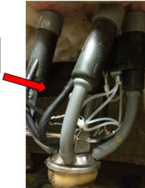
Fig.6; Air hoses are in good condition with no cracks or holes where vacuum leaks may occur.
