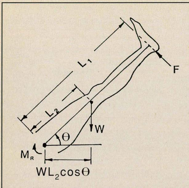
**Figure 1.** Free body diagram illustrating biomechanical model described in equation 1.  $M_R$  = resistive moment about hip joint;  $F$  = force applied at heel;  $L_1$  = distance from hip joint to heel;  $W$  = weight of leg;  $L_2$  = distance between hip joint and leg's center of gravity, and  $\theta$  = angle of leg to horizon.
