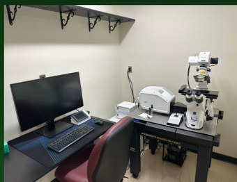
Figure 2. Confocal Imaging System and Analysis of OIR-induced Retinal Pathology. This illustrated the confocal microscope and its associated computer workstation used to acquire the are shown, illustrating the equipment used for retinal imaging.
