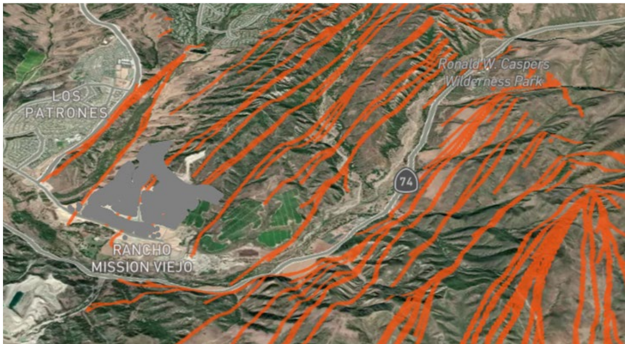
Fire pathways are drawn in orange on this image of RMV's PA3 study area. In this simulated wildfire event, the speed-based fire pathways are modeled during a Santa Ana wind event, with winds from the northeast. Source: XyloPlan. Map Data: ©2024 Mapbox.
