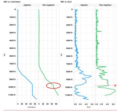
**Figure 1.** The maximum dogleg severity for the well with the Agitator and RSS was lower than the dogleg severity for the well without the Agitator for a similar well profile. As shown here, the conventional BHA had more difficulties steering, resulting in unplanned high doglegs and, consequently, increased well tortuosity and poor hole quality.
