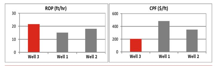
**Figure 3.** On the first offset well, ROP was 15.1 ft/hr, and on the second, it was 18 ft/hr. Based on the number of bits used and time downhole, the CPF for the first well was 483.3/ft, and it was 349.3/ft for the second. With the addition of the Agitator system and MOCS, ROP increased to 21.5 ft/hr, and CPF decreased significantly to 204 ft/hr.
