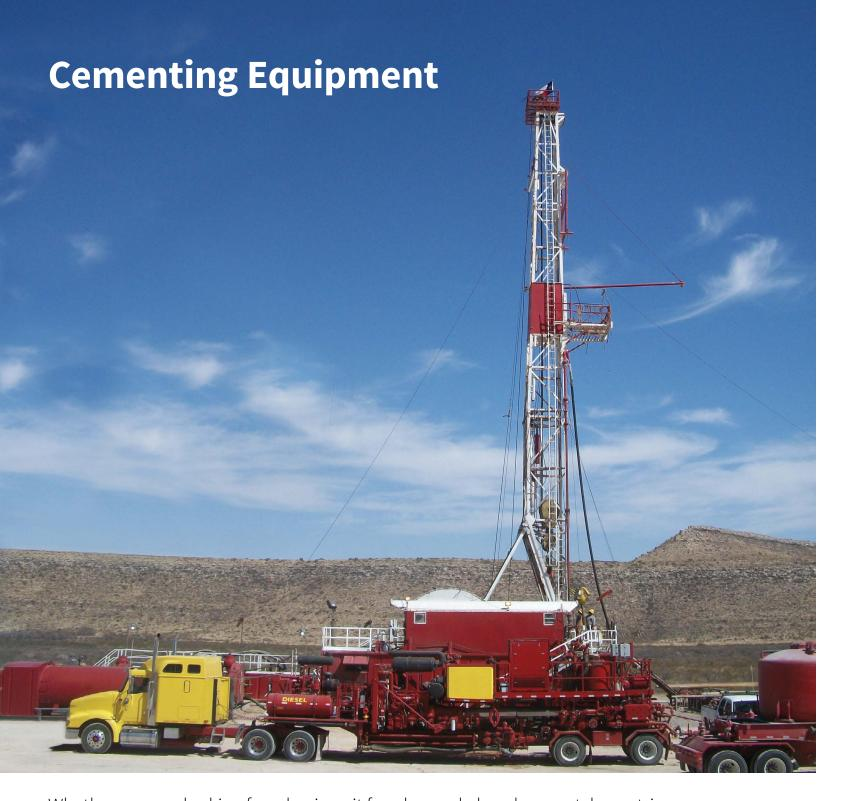
Whether you are looking for a basic unit for plug and abandonment, long string horizontal casing or offshore high horsepower, we manufacture units to meet your cementing requirements. Our units provide precise management of the cement mixing and pumping process to ensure successful completion.
