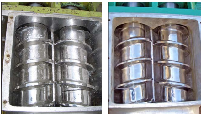
These before and after photos show how used feed screws can be returned to like-new condition.
