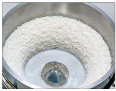
particles is time and formulation dependent. Once the desired particle shape is achieved, the batch is discharged through a manual plug valve and discharge chute, collected, and dried.
