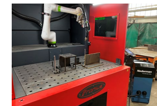
On-torch fume extraction for cobot workstation with FE GoMax
