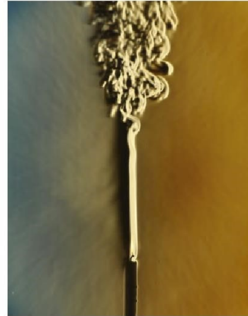
(c) Candle flame and smoke showing transition from laminar to turbulent flow.
