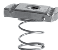
Channel Nut with Short Spring, an accessory to Universal Brackets. Order separately. Length: 24 mm, Height: 4 mm, Weight: 0,03 kg.
