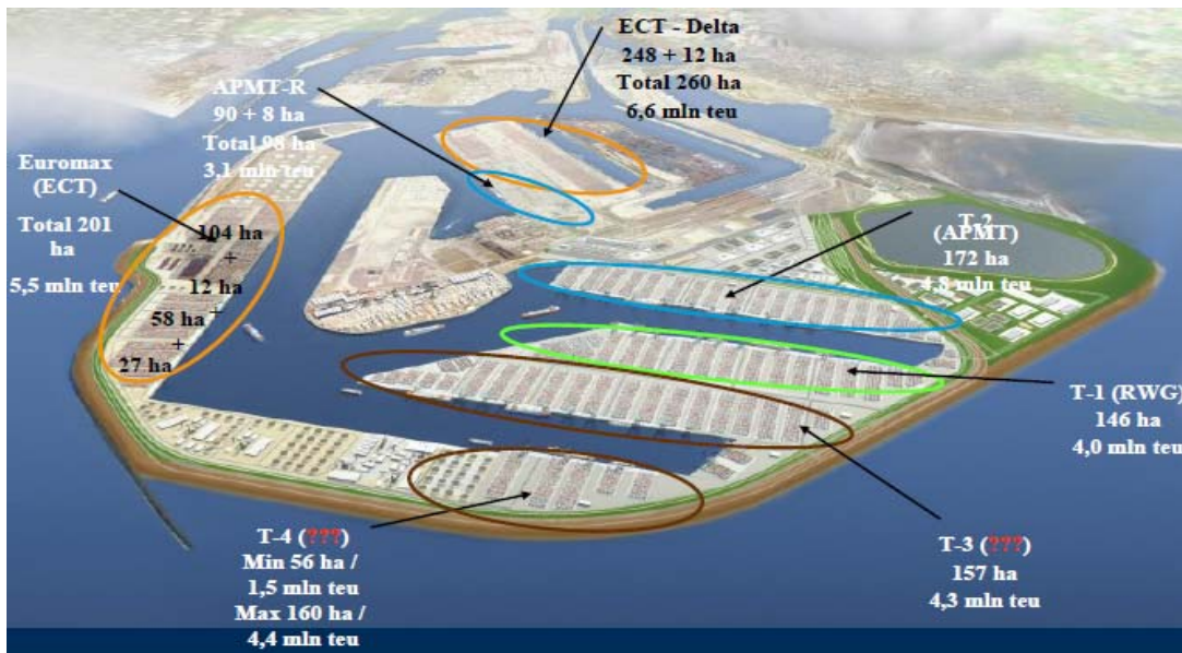
Source: Port of Rotterdam Hinterlands Project, Donald Baan, June 2009 Figure 28: Rotterdam Maasvlakte Container Port
