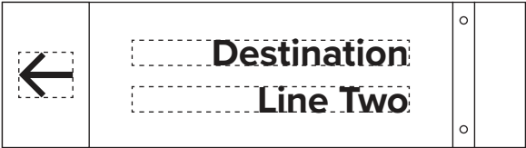
3 SIGN TYPE D1 - ELEVATION, DOUBLE-LINE (DESTINATION WITHOUT MILE INFORMATION) 1"=1'-0"
