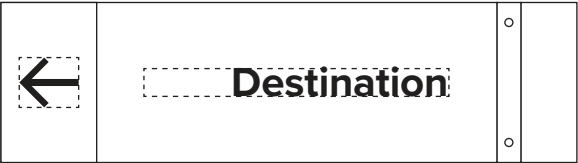
4 SIGN TYPE D1 - ELEVATION, SINGLE-LINE (DESTINATION WITHOUT MILE INFORMATION) 1"=1'-0"
