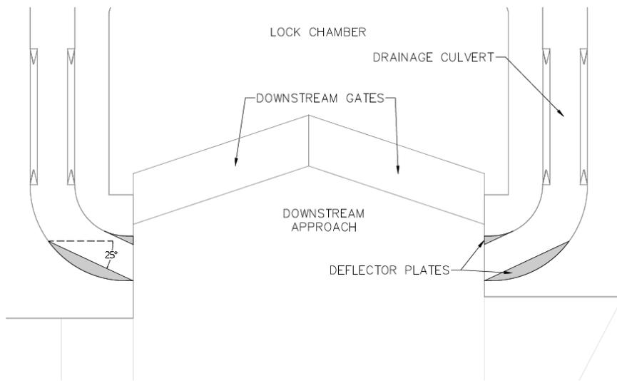
Preliminary simulation results showed low velocities in the area between the culvert openings and the downstream gates. Therefore, modeling was also completed for a scenario where outlet flows were directed upstream using discharge deflectors. The upstream deflection geometry shown in Figure 6 used a 20-degree upstream deflection.
