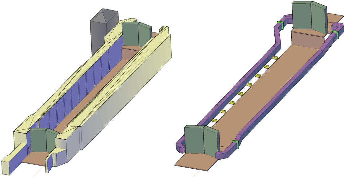
Modeling was also completed for a scenario where outlet flows were directed downstream using discharge deflectors. The modified culvert openings were designed to smooth flow and reduce turbulent discharge patterns from the existing outlet geometries. Anchor QEA modeled deflector plates that redirect flow 25 degrees downstream. Figure 5 shows the modified culvert openings, with the deflector plates shaded gray.
