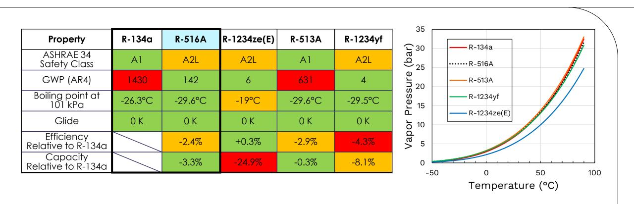
→ R-516A provides matching thermodynamic properties and cycle performance to R-134a making it an ideal design compatible replacement for both heating and cooling applications
