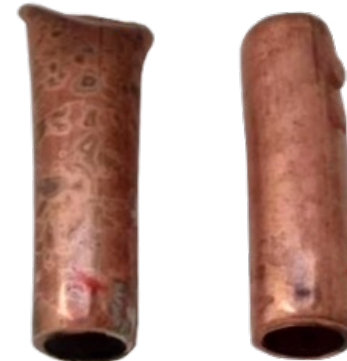
Unprotected pipe sections
