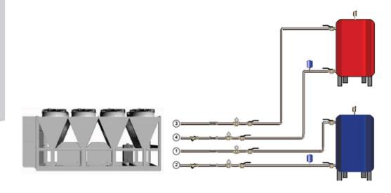
The SILVER range chillers installation, for the version with total heat recovery option, includes two inertial water tanks too. The blue tank (cold) is dedicated to the main users circuit, the chiller works to keep the inertial tank at the needed temperature using the chiller inlet water temperature to regulate the cooling capacity.
