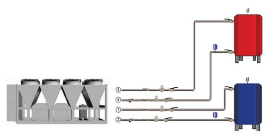
The SILVER range chillers installation, for the version with desuperheater option, includes two inertial water tanks too. The blue tank (cold) is dedicated to the main users circuit, the chiller works to keep the inertial tank at the needed temperature using the chiller inlet water temperature to regulate the cooling capacity.
