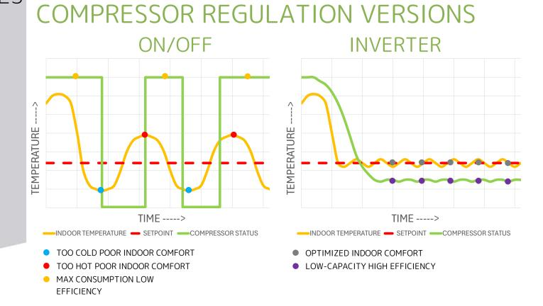
SILVER RANGE IS ALWAYS COMPLETE WITH INVERTER REGULATION ON ONE OR TWO COMPRESSORS.
