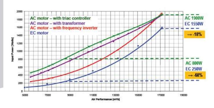
As shown in the chart, at half of the maximum airflow (low fan speed), the energy savings can reach up to 68% compared to an AC Fan.At maximum airflow (high fan speed), the energy savings remain an impressive 18% compared to an AC Fan. Fans are rarely used at maximum speed, so the energy savings allow you to recoup the cost difference of EC Fans within a few months. On average, fans operate at half of the maximum airflow, resulting in energy consumption reductions of 43% to 50%
