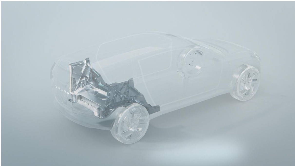
At Volvo in Torslanda, a considerable proportion of the rear vehicle floor is to be cast in one piece.
