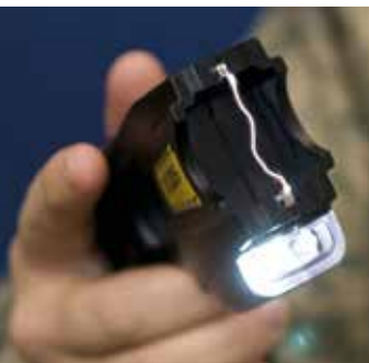
The electronic control devices used by security forces at Grissom Air Reserve Base, Indiana, deliver a high-voltage, low-power charge of electricity to disrupt a person's central nervous system and induce involuntary muscle contractions. (Photo: Technical Sergeant Mark Orders-Woempner)
