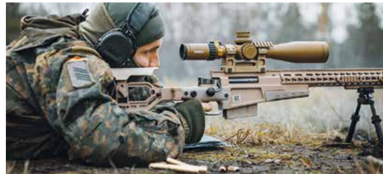
Left: The G22A2 sniper rifle is a repeating rifle with a calibre of 7.62mm. It weighs nine kilograms and has a sight with a magnification factor between 3 and 12. Right: Five cartridges fit into the magazine of the G22A2 rifle and must be manually reloaded by the shooter. (Photos: Bundeswehr/Maximilian Schulz)
