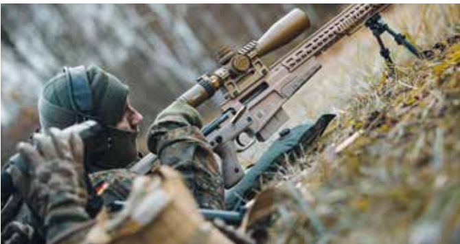
Left: The G22A2 sniper rifle is a repeating rifle with a calibre of 7.62mm. It weighs nine kilograms and has a sight with a magnification factor between 3 and 12. Right: Five cartridges fit into the magazine of the G22A2 rifle and must be manually reloaded by the shooter. (Photos: Bundeswehr/Maximilian Schulz)
