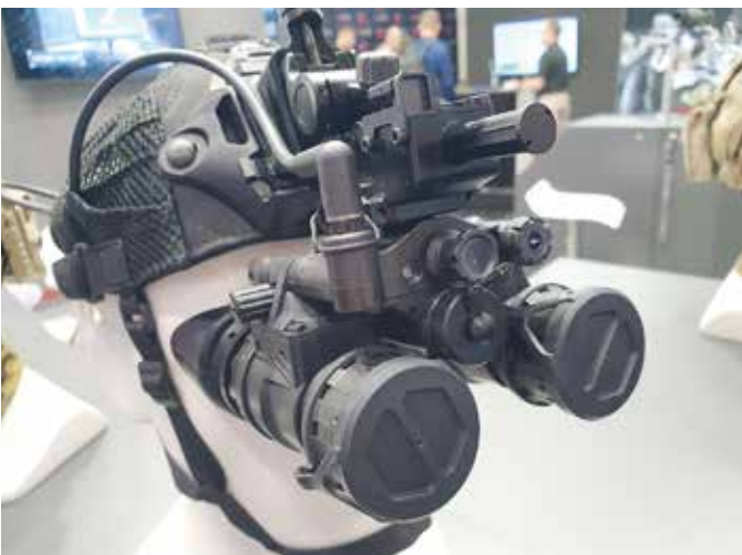
Left: Belgium and Germany rely on THEON Sensors' MIKRON binocular night vision goggles with two 16mm image intensifier tubes and an integrated infrared illuminator. Right: Widely in operational use: MIKRON binocular with 18mm image intensifier tubes. (Photos: Stefan Nitschke)
