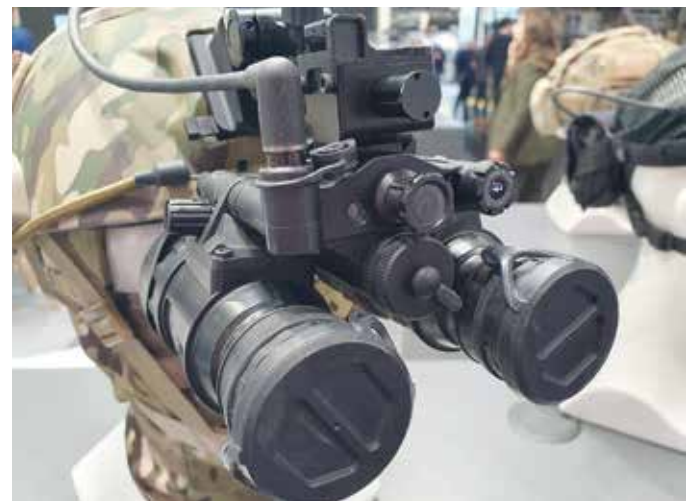
Left: Belgium and Germany rely on THEON Sensors' MIKRON binocular night vision goggles with two 16mm image intensifier tubes and an integrated infrared illuminator. Right: Widely in operational use: MIKRON binocular with 18mm image intensifier tubes. (Photos: Stefan Nitschke)
