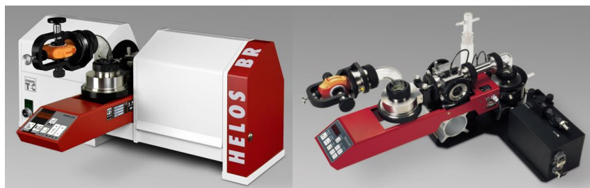
Fig. 1: (left) Laser Diffraction system HELOS/BR + dispersing system INHALER; (right) INHALER with Dry Powder Inhaler (DPI) device (orange) adapted in front of the 90° glass pipe bend (as simulation of the throat).
