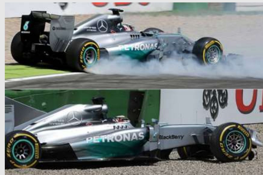
German GP 2014, brake disc failure causes crash
