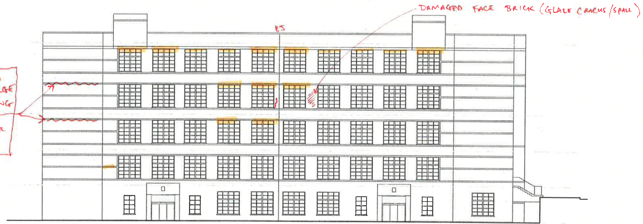
EAST ELEVATION DAMAGE MAP
