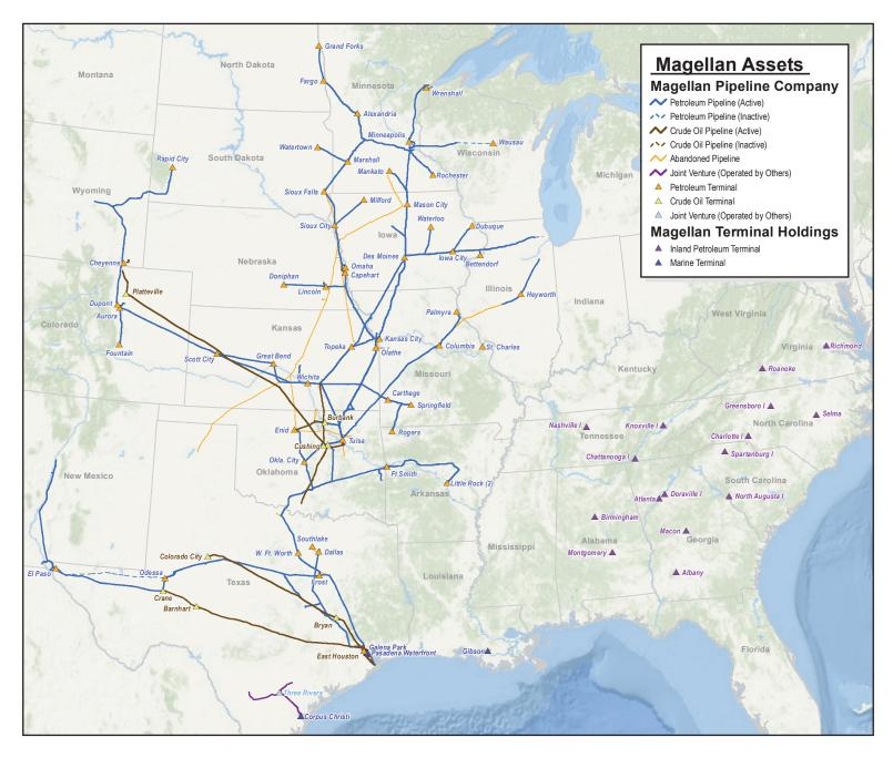
Magellan is the longest common carrier pipeline system for refined products and liquid petroleum gases (LPGs) in the United States, extending approximately 9,800 miles from the Texas Gulf Coast and covering a 15-state area throughout the central U.S. The system includes 54 connected terminals and 25 independent terminals. Magellan also owns and operates over 2,200 miles of crude oil pipelines with over 37 million barrels of storage.
