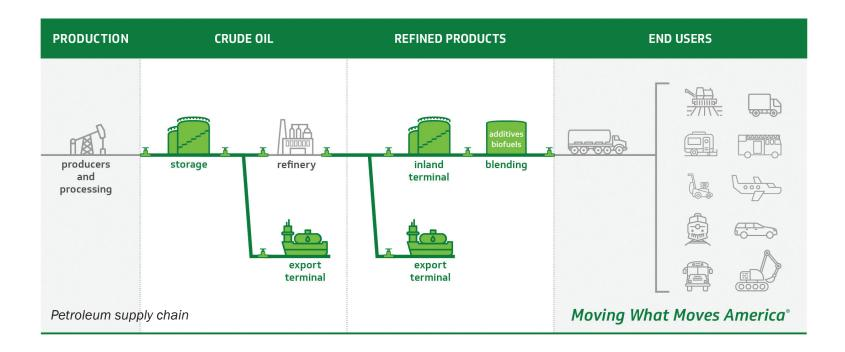
At the refinery, crude oil is processed into various petroleum products, including gasoline, diesel fuel, jet fuel, and more. Those products are then transported via pipeline to a refined products terminal where they are segregated further, tested for quality, and readied for distribution. Transport trucks complete the final step of delivering these products to a neighborhood service station.
