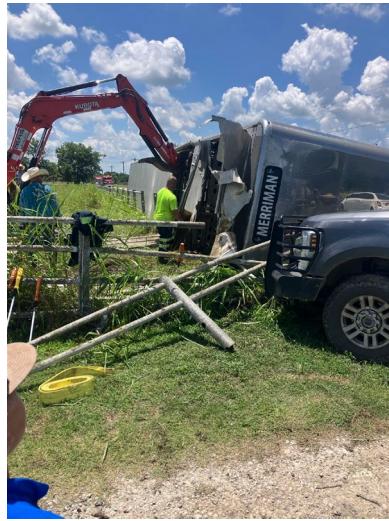
Wrecker company uses excavators to pry the overturned trailer open.
