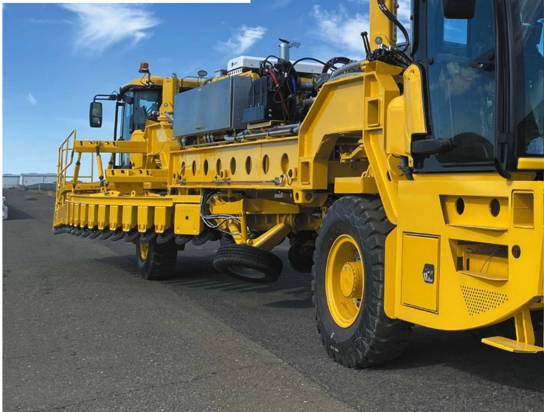
Above: The barrier transfer machine transferring the barrier by one lane
