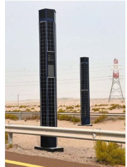
Left: Traffic safety solution (TOTEM) Right: Solar Intelligent Speed Enforcement Radar (ISER)
