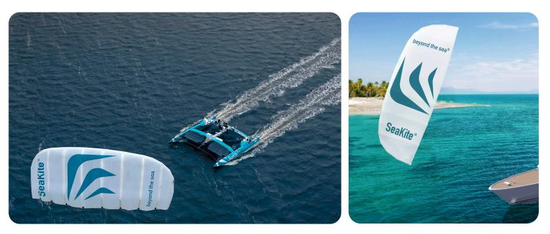
Beyond the Sea has developed **SeaKite**<sup>®</sup>, an innovative and **fully automated kite traction system** designed to **reduce fuel consumption** and make maritime transport **more sustainable**. This environmentally **friendly technology** combines a kite, a launch mast, electronic sensors, a KiteBox (featuring winches and autopilot), and an intuitive human-machine interface.
