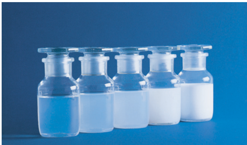
Figure 2: Translucent to opaque boehmite sols, each with a concentration of 10 wt.% AlOOH
