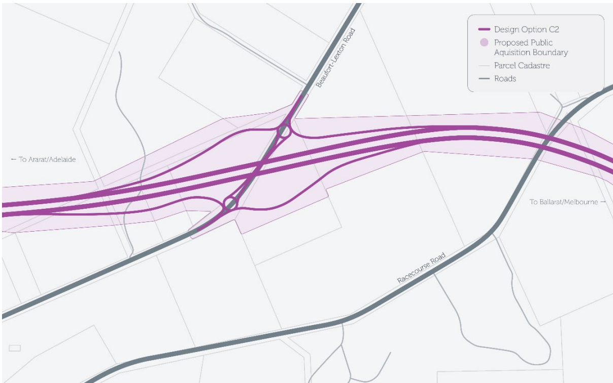
Figure 4.8 Project access arrangements – Beaufort-Lexton Road interchange
