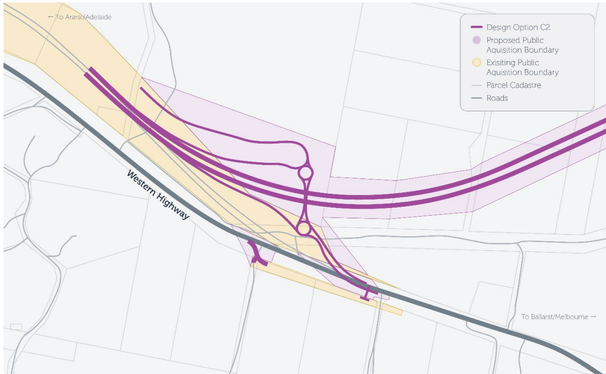
Figure 4.7 Project access arrangement – western tie in
