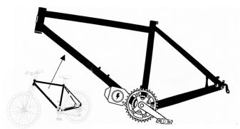
Motors are only permitted if they are housed <u>within</u> the frame or wheel. Attachments outside of the frame that drive the pedals (mid-drive conversion) or to the back wheel (prepackaged) are converted e-bikes.
