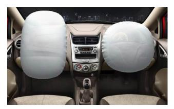
People inside a car are better protected in the event of a crash due to modern vehicle features—such as front, side and curtain airbags. All new cars since 2011 have electronic stability control (ESC) which can help to avoid a crash.
