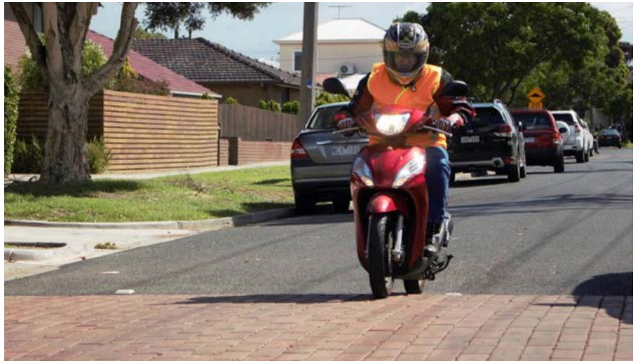
A simultaneous change in surface type and surface height can result in a motorcycle losing traction.
