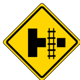
Uncontrolled rail crossing on side road sign
